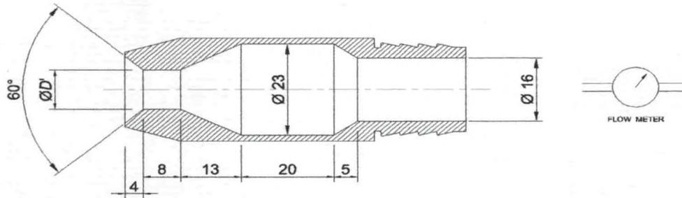
$\phi D' = 6,3$  mm unit: mm
